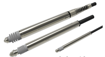
8, 6 and 3 mm diameter probes
