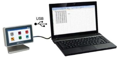
The M1 and M3 hardware are configured as a USB keyboard. When the displays are connected to a computer with USB, it is automatically detected as an additional keyboard.
