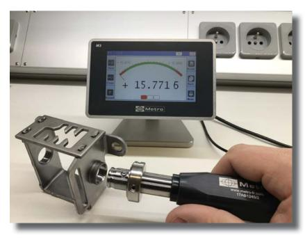
16N7 Internal diameter measurement on a air plug gage directly connected on a M3 display
