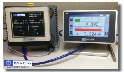
Communication between a M3 display and a Proface PLC with the Modbus RTU protocol. The HMI from Proface has been programmed with differents buttons and indicators allowing to control and bring back informations from the M3.
