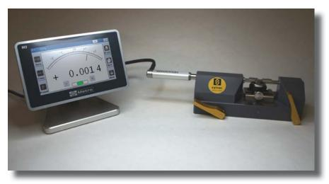
Measurement of very small watch parts. Here the M2 is connected with a Heidenhain SPECTO probe, mounted on a Sylvac PS15 measuring bench.
