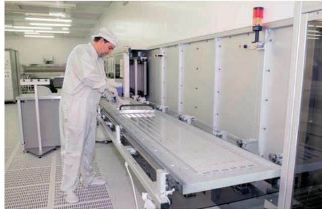
Vacuum machine for application of chromium layers
