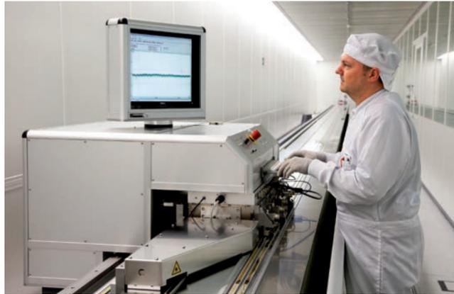
30 m long measuring machine for scale tapes
