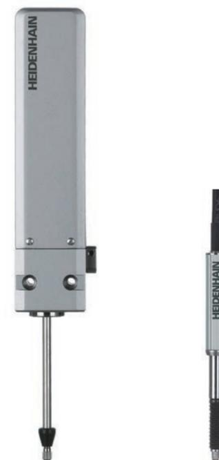
With **incremental linear encoders**, the current position is determined by starting at a reference point and counting measuring steps, or by subdividing and counting signal periods. Incremental encoders from HEIDENHAIN feature reference marks, which must be scanned after switch-on to reestablish the reference point. This process is especially simple and fast with distance-coded reference marks.
