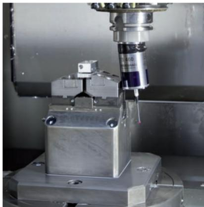
Touch probe with **radio and infrared transmission** for machines with automatic tool change:
