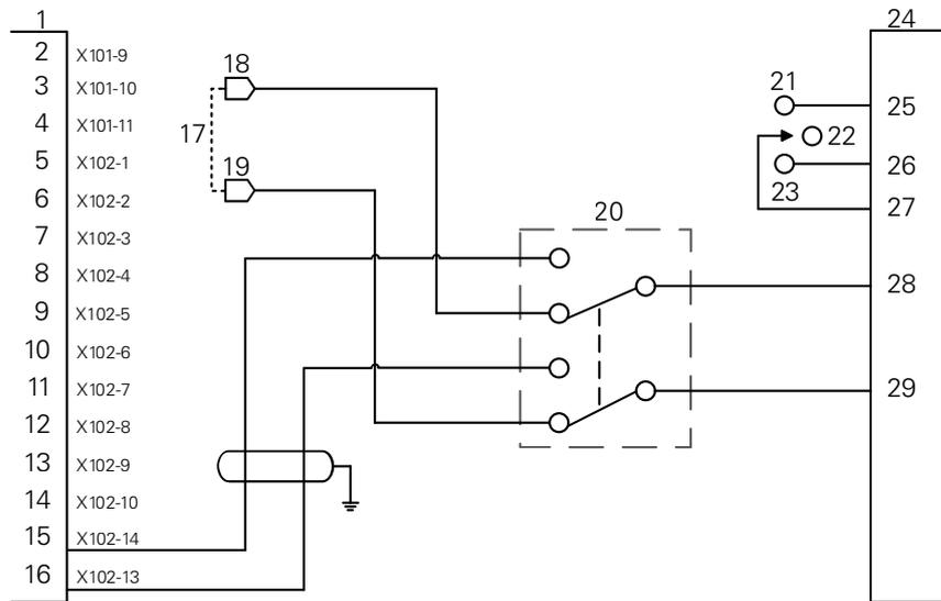
Example of switching to manual spindle speed control
