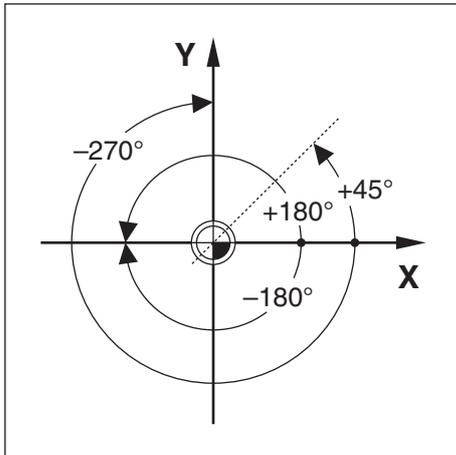
The Zero Angle Reference Axis is the  $0.0^\circ$  position. It is defined as one of the two axes in the plane of rotation. The following table defines the Zero Angle where the position of the angle is zero for the three possible planes of rotation.
