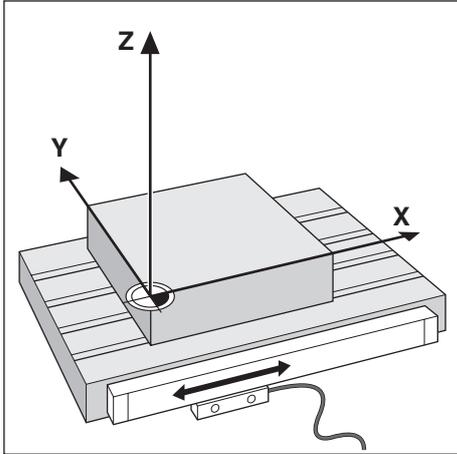
The reading head position provides feedback to the product that converts the movement of the machine axes into electrical signals. The product constantly evaluates these signals, calculates the actual positions of the machine axes, and displays the positions as a numerical value on the display.
