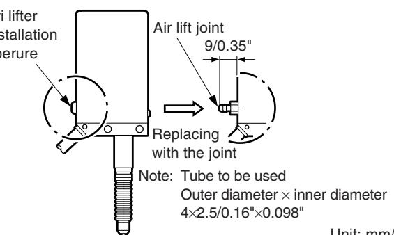
Fig. 2. Using the air lifter (DL310B)
